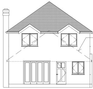
Lines indicating eaves height of original bungalow. Eaves height to be no higher than this line in accordance with permitted development conditions. Top of mono pitch roof to finish lower than ridge height of original bungalow as per permitted development conditions.
